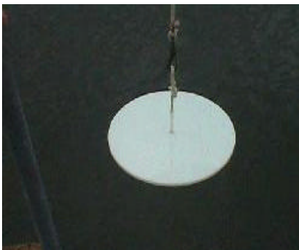
A Secchi disk just below the water surface, on its way down to check water clarity
